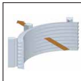
Internal Circumferential Wire Construction
